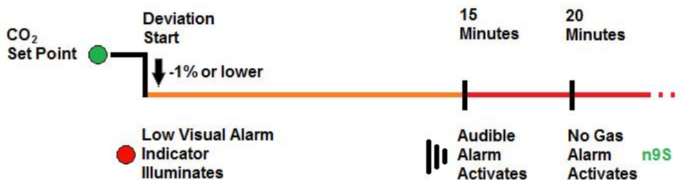
Low and No Gas Alarms Timeline
