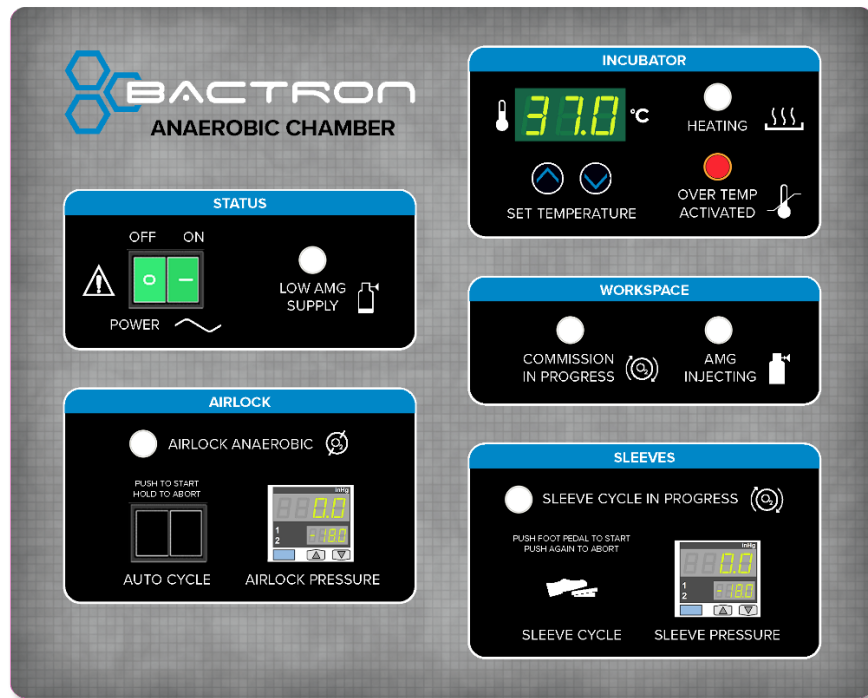
Figure 8: Main Control Panel
