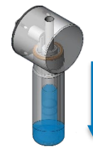
Water in the manometer outer bottle forced down
